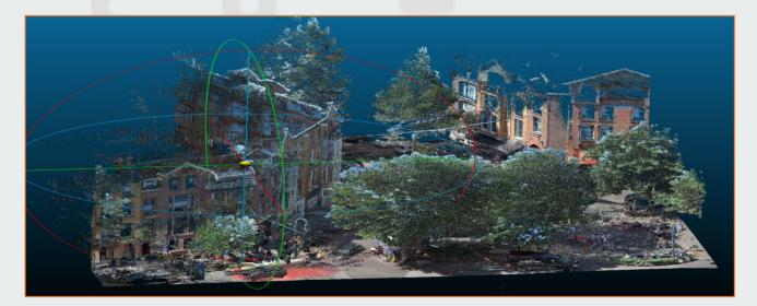
Ground Segmentation: The CSF (Cloth Simulation and segmentation) plugin was utilized
