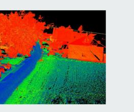
Tree Isolation: The TreeIso plugin was employed to isolate individual trees within the point cloud. This plugin utilizes advanced algorithms to detect and segment trees.
