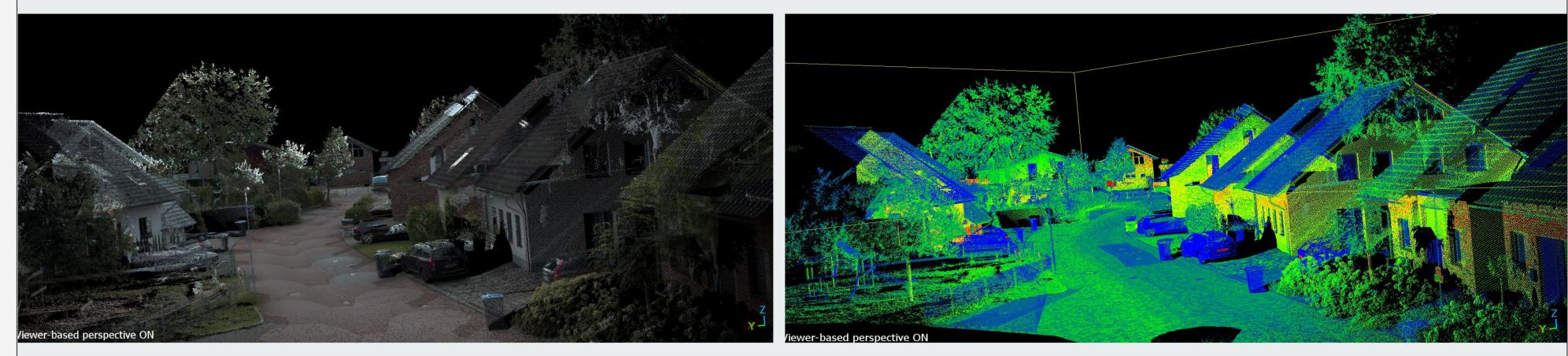
Point cloud data represents a collection of 3D points in space, often obtained from laser scanning or depth sensors, providing a detailed representation of surfaces or objects.
