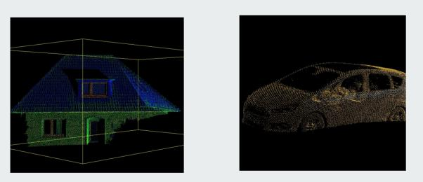
Connected components segmentation was applied to identify and label distinct objects within the point cloud, such as cars, houses, and roads. This process involves grouping adjacent points with similar properties to form coherent objects. Labeled points are used to generate a new LAS file, where each point is assigned a specific class. This labeled LAS file can be further processed, including training classification model and segmentation model.
